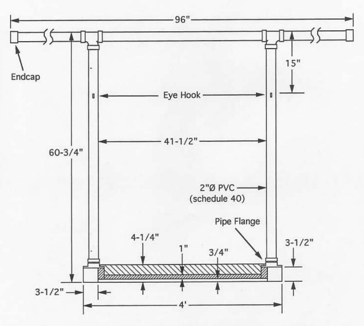
Notes: Nylon rope and lower eye hooks and omitted for clarity.
